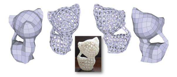
Figure 1: A nearly symmetric quadrangular mesh generated using the operator based representation of vector fields (Azencot et al., 2017) (left and right). The symmetry enables the generation of a very low resolution model, which can be fabricated using additive manufacturing, by thickening the quad mesh edges (left center and right center). The center image is a photograph of the final printed model.
